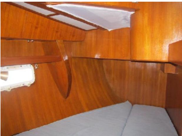
Ventilation via two ports and overhead hatch
